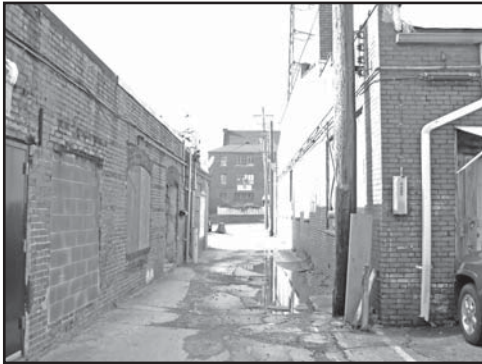
Service areas and alleys shall be maintained clean of debris and standing water. Inadequate drainage can cause infestation, as well as water damage, to buildings given the nature of their use for the placement of dumpsters and recycling bins.
