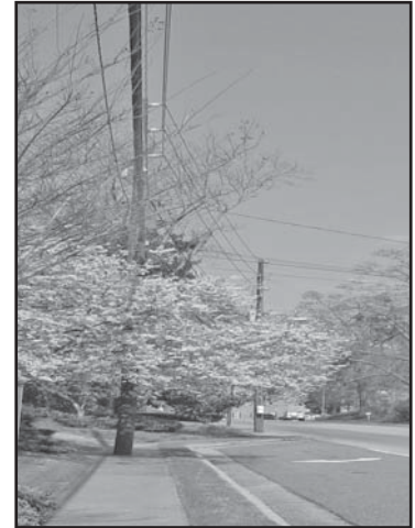
This planting strip of approximately 18” provides a psychological buffer for a pedestrian from oncoming traffic. Such planting strips are required whenever feasible.
