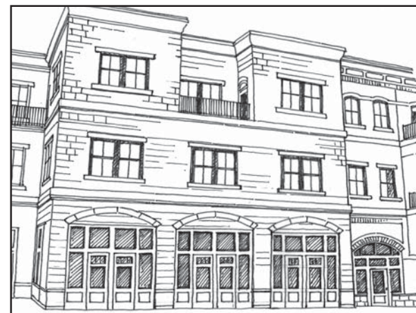
This sketch depicts multi-story development that is high density and mixed-use with commercial storefronts on the first floor with offices, or apartments on the second floor. The character of this building is commercial and would be appropriate for a project located in the historic commercial core of Main Street between Lewis Street and Watts Drive.
