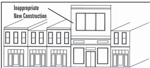
The above new construction is out of scale to the adjacent two story constructions.
